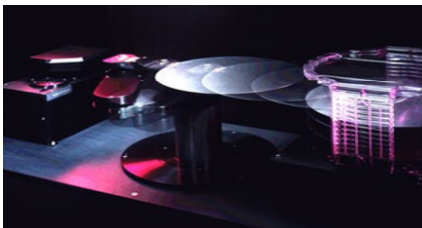
Cassette-to-cassette robotic handling provide completely automated measurement
